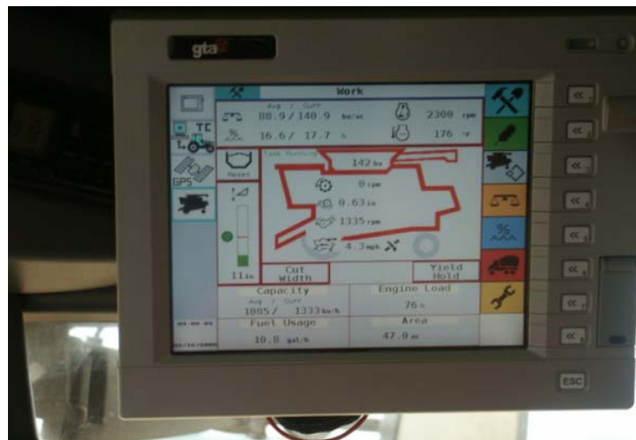
Figure 6. Example yield monitor display mounted in the combine cab.
