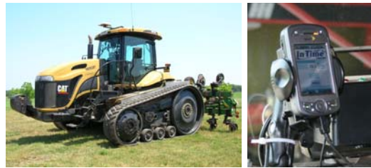
Figure 1. Tractor equipped with RTK GPS receiver and internet accessible cellular phone which receives real-time GPS correction signal from a CORS site in
