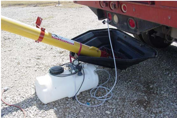
Calibrating a sprayer used to apply grain protectant
