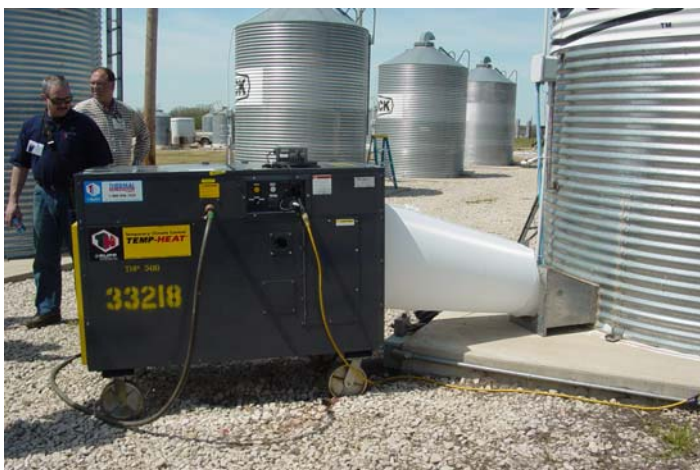
Apparatus for applying a heat treatment to stored grain
